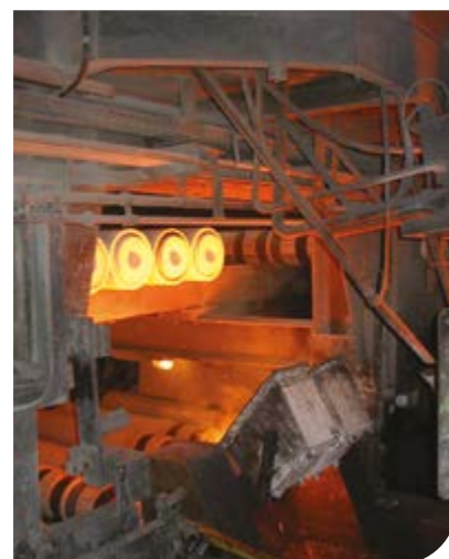
Centrifugal casting process
