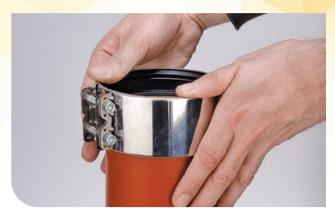
2. Ease-in one side (next to the continuity spur) then push down on the opposite side of the coupling to fully seat, ensuring that the central inner register is abutted against the spigot end.
