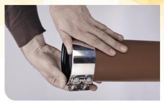
Ease-in one side (next to the continuity spur) then push on the opposite side of the coupling to fully seat, ensuring that the central inner register is abutted against the spigot end.
