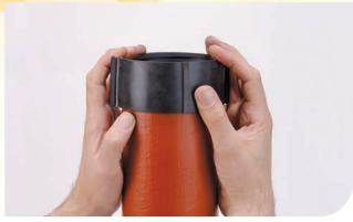
Push the EPDM rubber gasket over the end of the pipe or fitting, ensuring that the central inner register is abutted against the spigot end.
