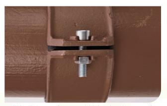
6. All Ductile Iron couplings use an M8 bolt and require a 6mm allen key. The coupling incorporates an anti-turn feature which holds the bolt nut in place without the need for a secondary tool. (See page 47 and 59 for details of fixing tools)
