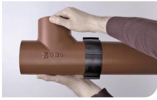
3. Ease the next pipe or fitting into the EPDM rubber gasket making sure that the spigot end is against the central inner register.
