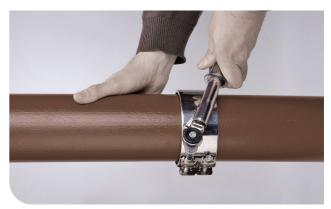
Evenly tighten the bolts to the required torque setting. The coupling should only be tightened once, because it cannot be dismantled and re-used. (See Couplings Data page 55)
