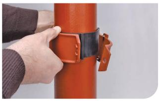
4. Loosely fit the coupling around the gasket, ensuring that the rubber lip sits into the corresponding locator in the coupling. The electrical continuity screws should be drawn back to fullest extent to avoid interference with the connecting pipe or fitting.
