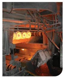
Centrifugal casting process
