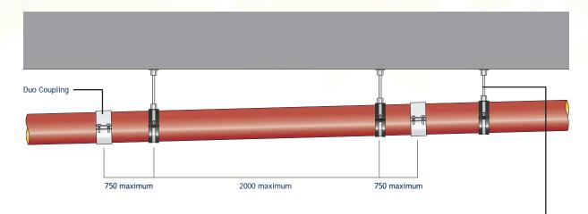
It is recommended that each pipe length in a horizontal pipe run should be supported by 2 brackets, not more than 2m apart. The length of pipe between a bracket and a coupling should not exceed 750mm.
