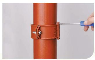
For electrical continuity, hand-tighten the electrical continuity screws on both sides. Ensure screws pierce external coating of pipe when tightened. (See page 55)
