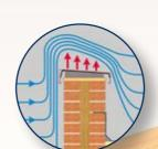
When tested under extreme loads, Skyline Coping System met the required test standard of 6kPa (220mph) under static load conditions
