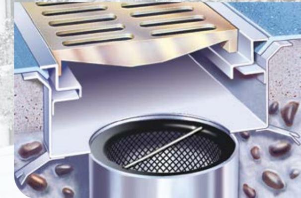
Typical installation in a vinyl covered floor SN12230 grating with SVFB channel. Channel profile SVF ensures watertight connection when used with flexible sheet material such as vinyl flooring. Suffix 'B' on channel Spec. Code denotes filter bucket.
