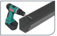
2) Drill Ø8mm holes, 18mm from the top edge of the gutter at 900mm centres and a minimum of 50mm from the ends of the gutter
