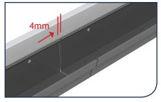
5) When joining gutter lengths, allow for a 4mm expansion gap.
