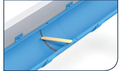
9) Tool-off displaced silicone sealant from the newly formed gutter joint. Allow to cure for 24 hours
