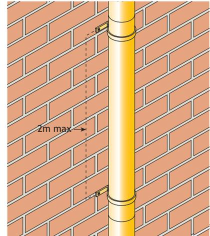
Pipe clips support and hold the rainwater pipe to the structure. All three types of pipe clip, Standard, Small Base and Extended Base can be used to conceal the pipe joints.
