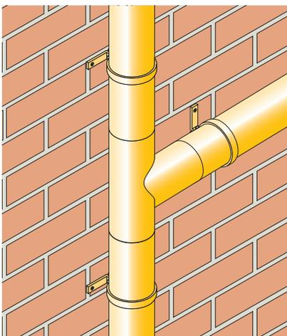
Continue to assemble the stack taking care not to scratch the pipe coating whilst sliding pipe clips into position.
