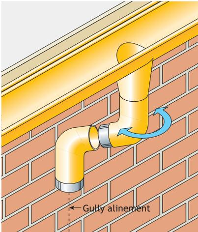
Check alignment of gutter outlet to gully. Where square or rectangular pipes are being installed and offsets are required, alignment between the gutter outlet and gully must be exact.
