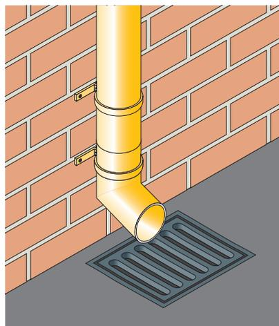
At ground level if the rainwater pipe does not connect directly to the gully, pipes can terminate with a shoe fitting for free discharge over the gully.
