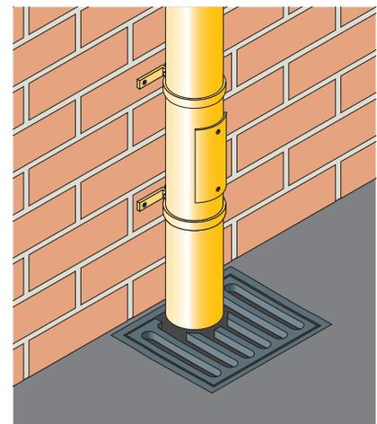
Where rainwater pipes directly connect to the gully it is recommended that an access pipe is fitted no more than 750mm above ground level.
