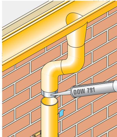
Commence installation from the gutter outlet by fitting and adjusting the two part offsets. Check vertical plumb line and assemble internal spigot joints using DOW 791 silicone sealant then fit first pipe clip.
