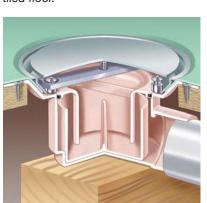
Watertight trapped drainage in a vinyl covered timber floor.
