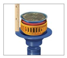
Prior to installation, check height of components to ensure compatibility with roof build-up, making allowances for the membrane thickness.
